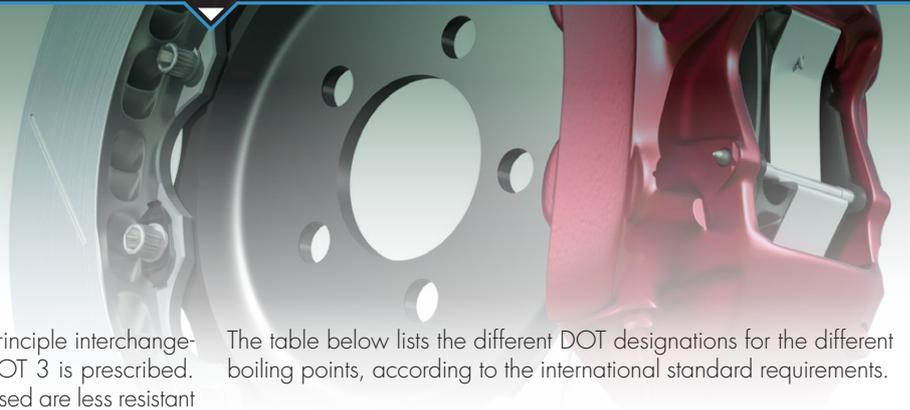
Brake fluids based on polyglycol ethers are in principle interchangeable. However, it may be that specifically a DOT 3 is prescribed. Most often this is because the sealing materials used are less resistant to the DOT 4 brake fluid.
